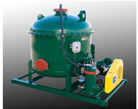
The Degasser is effective in removing entrained gas, but it can only process part of the drilling fluid returns passing through the Desander, which means that some of the gas-cut returns will reach the Desilter Tank and remain untreated.
