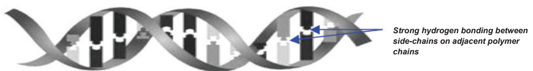
Figure 7: Double Helix Structure of Xanthan Gum in Solution.
