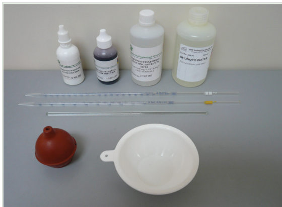
Equipment used for measuring Total Hardness as Calcium.
