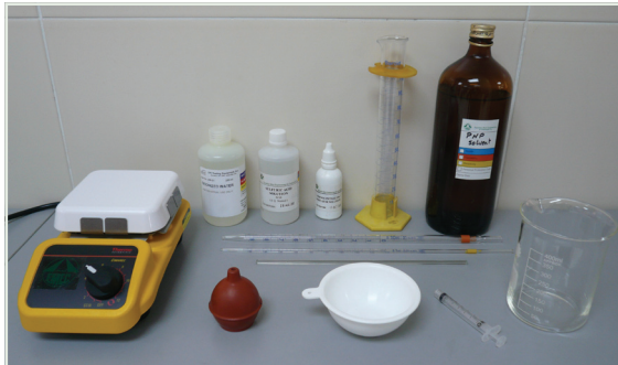
Equipment used for measuring Whole Mud Alkalinity and Lime Content.
