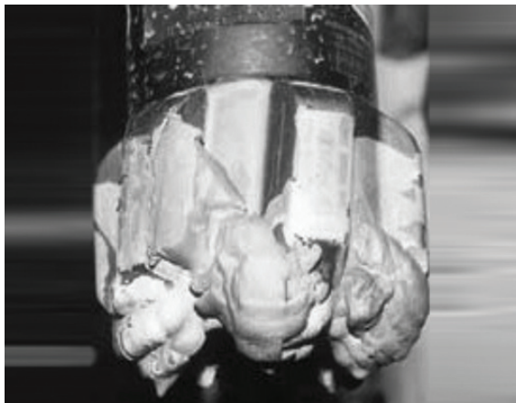
An example of bit-balling.
