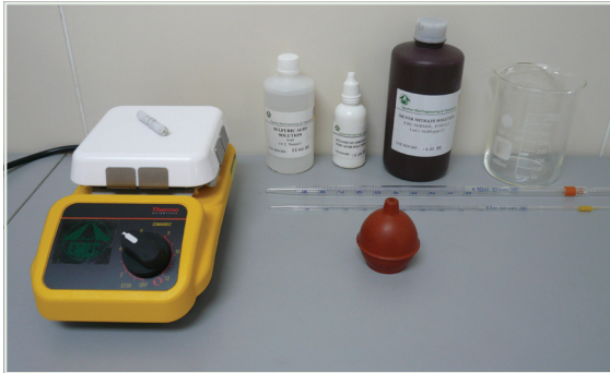
Equipment used for measuring Whole Mud Chloride Content.
