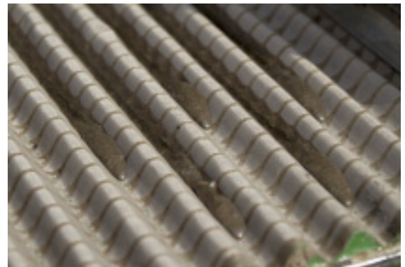
Cuttings being removed by the shale-shaker screens
