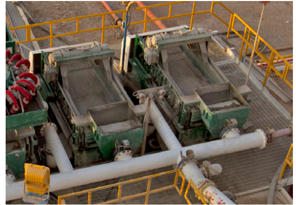
A Pair of Shale Shakers
