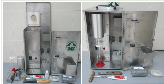
Retort Kit before and after assembly
